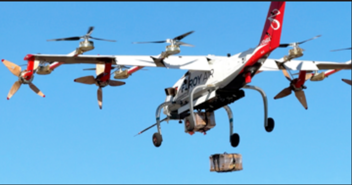
THE HYBRID-EVTOL CHAPARRAL UAS IS UNIQUELY DESIGNED TO MOVE SUBSTANTIAL VOLUMES OF CARGO BY AIR BETWEEN FLEXIBLE LOCATIONS WITH MINIMAL INFRASTRUCTURE.
